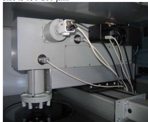
Fig.1: Opto-mechanical unit for process monitoring and on-line control of the SLS machine.
