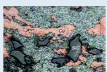
Cu+Al+SiC coating on steel substrate Initial composition of the mixture: 30%Cu - 40%Al - 30%SiC
