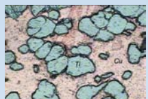
Ti+Cu coating on steel substrate Initial composition of the mixture: 50%Cu - 50%Ti
