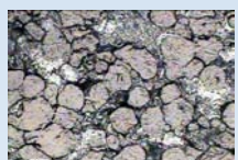
Ti+Al coating on steel substrate Initial composition of the mixture: 30%Al - 70%Ti
